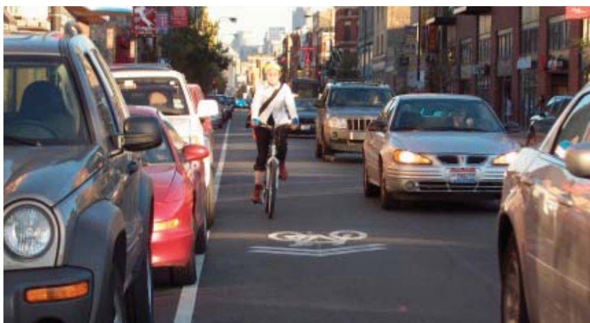
Figure 3.4-7 Partial Sharing for Bicycles and Motor Vehicles
