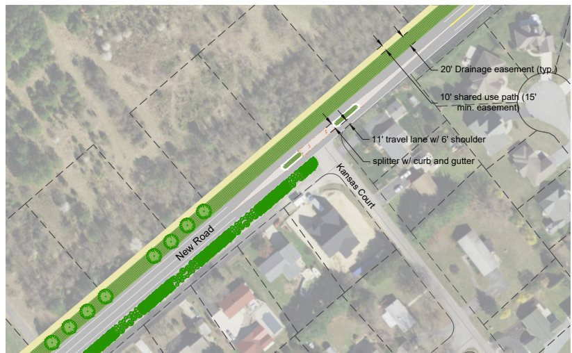
SPLITTER ISLAND AT KANSAS COURT
