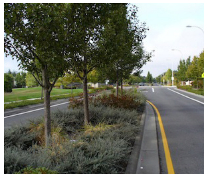
Figure 81 12' splitter island with turn lane
