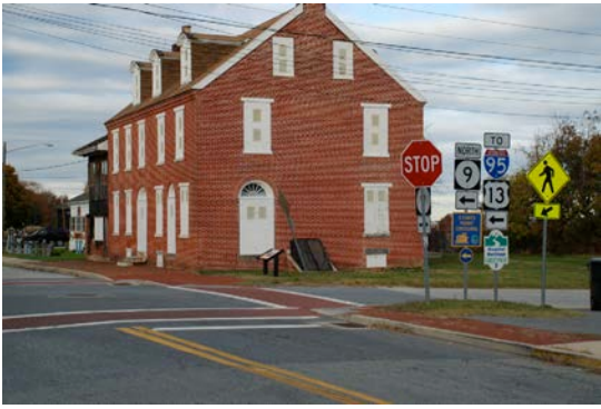
Figure 62 Excessive signage, such as the multiple sign panels on Delaware's Bayshore Byway at Port Penn should be avoided by coordinating directional signage and wayfinding, as well as keeping regulatory and advisory warnings to the minimum required
