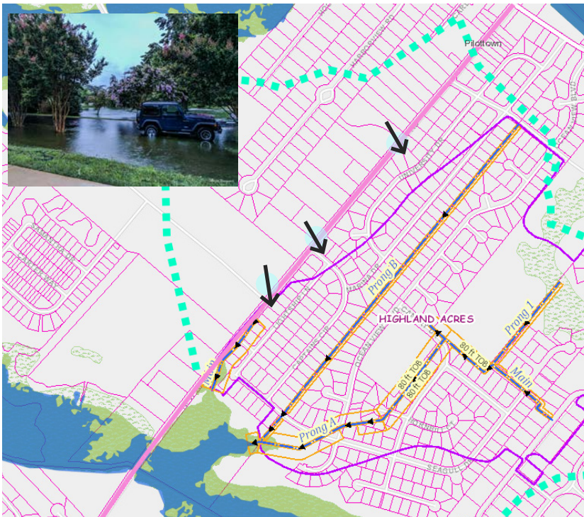
Figure 90 Catchment Area for the WB side of New Road feeds to culverts (blue circles)- NTS
