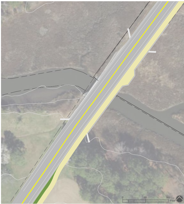
Figure 87 Illustrative concept showing a combined structure used to accommodate both the vehicular travel lanes and the shared use pathway with an overlook to Canary Creek
