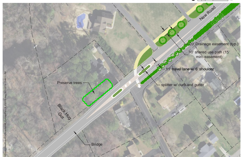
SPLITTER ISLAND AT ARKANSAS
