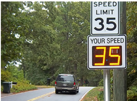
Figure 29 Multiple studies have shown that radar activated speed limit signs with changeable message reflecting actual speed are effective means of slowing operating speeds of between 3-8 mph (Source: FHWA)
