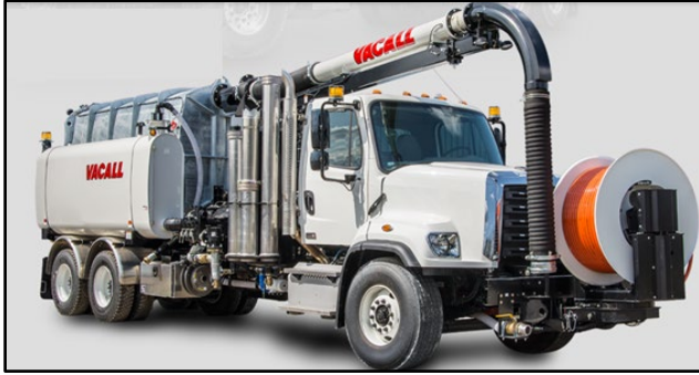
Combination Jetter and Vacuum Truck. Image Courtesy of Vacall Industries
