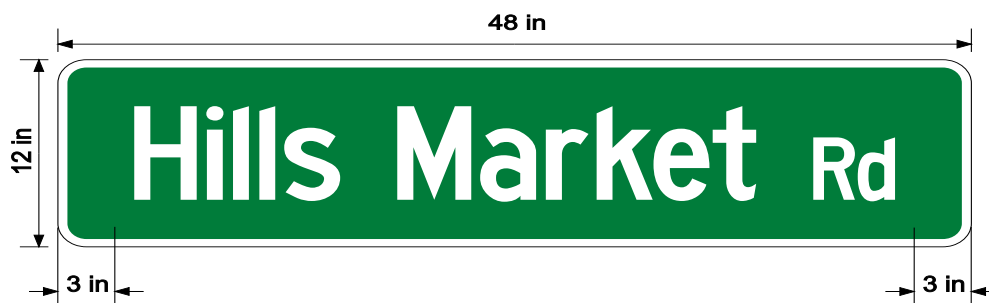
Figure 8. Panel size - 48"x12"; Legend- Highway C (6") for street names and Highway C (4") for type of roadway. Legend is center justified with normal letter kerning.
