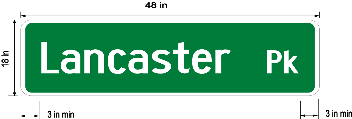
Figure 12. Panel size -48" x 18"; Legend- Highway C (8") for street names and Highway C (6") for type of roadway. Legend is center justified with normal letter kerning. Legend length is larger than 42".
