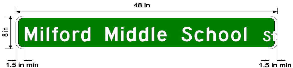
Figure 5. Panel size - 48"x8"; Legend- Highway C (4") for street names and Highway C (3") for type of roadway. Legend is center justified with narrow letter kerning.
