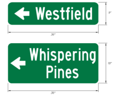
COLORS: LEGEND BORDER - WHITE (RETROREFLECTIVE) BACKGROUND - GREEN (RETROREFLECTIVE)
