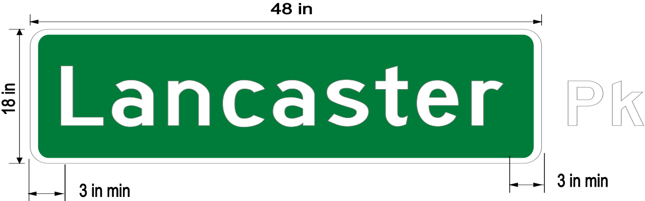
Figure 12. Panel size -48" x 18"; Legend- Highway C (8") for street names and Highway C (6") for type of roadway. Legend is center justified with normal letter kerning. Legend length is larger than 42".
