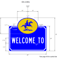
UPPER SECTION COLORS: LEGEND - BLUE (RETROREFLECTIVE) BACKGROUND - YELLOW (RETROREFLECTIVE) LOWER SECTION COLORS: LEGEND BORDER - WHITE (RETROREFLECTIVE) BACKGROUND - BLUE (RETROREFLECTIVE)
