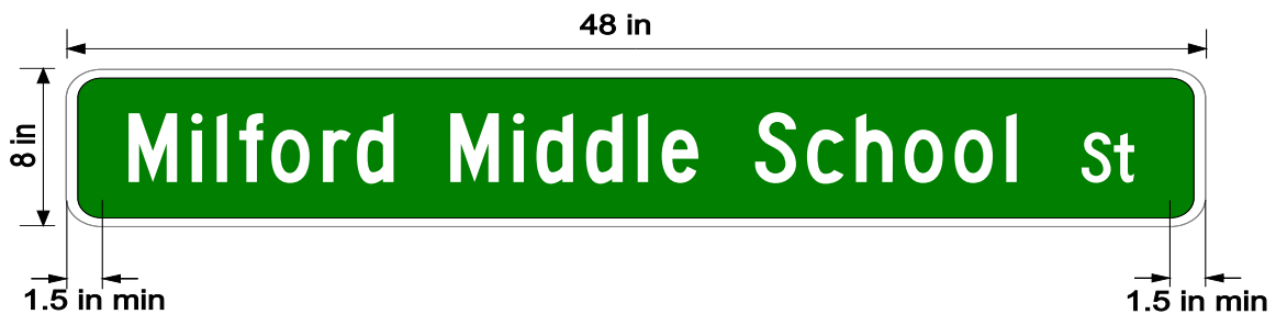
Figure 6. Panel size - 48"x8"; Legend- Highway C (3.5") for street names and Highway C (2.5") for type of roadway. Legend is center justified with narrow letter kerning.
