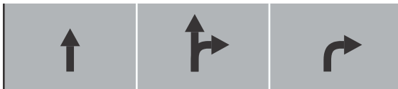
Figure IV-5k. One Through Lane, One Shared Through/Right Lane, and One Right-Turn Lane (Protected-Permissive Right-Turn Phasing)
