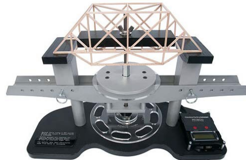
Figure 2. Pitsco Structures Testing Instrument
