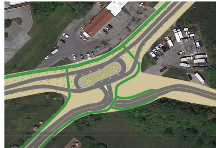
SR 9 / 6 th St at Chestnut St, New Castle, DE Proposed “Dutch Left” Conditions
