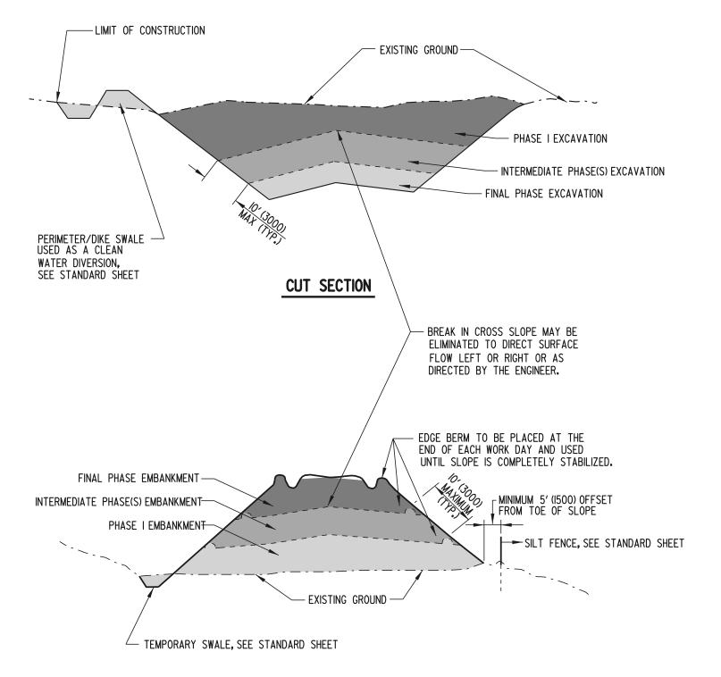
NOTES: I.) EDGE BERMS AND TEMPORARY SLOPE DRAINS SHALL BE CONSTRUCTED ALONG THE TOP OF ALL SLOPES TO INTERCEPT RUNOFF AND CONVEY IT DOWN THE SLOPE FACES WITHOUT CREATING GULLIES OR WASHOUTS.
