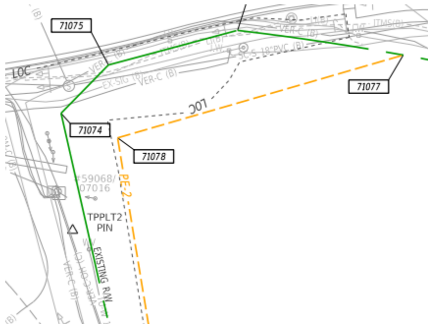
Figure 3-2 Limit of Construction within a Permanent Easement
