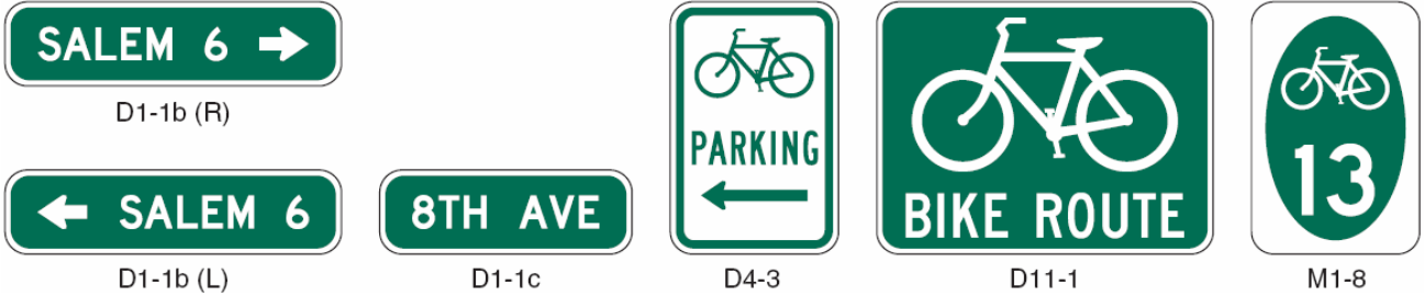
Figure F.3.1 Guide and Route Signs
