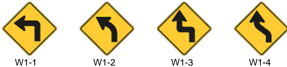
Figure F.2.1 Turn or Curve Signs Source: MUTCD, Figure 9B-3
