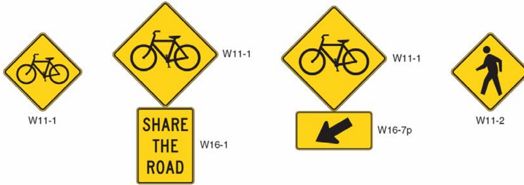
Figure F.2.6 Bicycle and Pedestrian Warning Signs Source: MUTCD, Figure 9B-3
