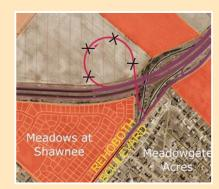
Removed northbound SR 1 loop ramp at Rehoboth **Boulevard to reduce property impacts**
