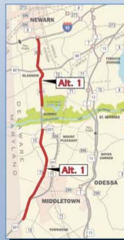
4 LANES - CONTROLLED ACCESS - NEW LOCATION ON ALIGNMENT
