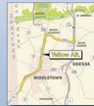
YELLOW ALT. 4 LANES - CONTROLLED ACCESS - ALONG EXISTING ROADWAYS New US 301 roadway along existing US 301 and existing SR 896 (Boyd's Corner Road)
