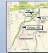
GREEN ALT. 4 LANES - CONTROLLED ACCESS - ON NEW LOCATION GREEN ALT. - OPT. 1 New US 301 roadway, west of existing US 301 (Ridge Alignment) then northeast from Armstrong to SR 1 south of C&D Canal GREEN ALT. - OPT. 2 New US 301 roadway, west of existing US 301 (Ridge Alignment), then northeast from Armstrong to SR 896, then north to new East-West Connection, south of C&D Canal
