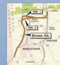
BROWN ALT. 4 LANES - CONTROLLED ACCESS - ON NEW LOCATION BROWN ALT. - OPT. 1 New US 301 roadway on new location, west of existing US 301 (Ridge Alignment) and East-West Connection, south of C&D Canal BROWN ALT. - OPT. 2 New US 301 roadway on new location, west of existing US 301 (Ridge Alignment) and North-West Extension through Summit Airport, then along new East-West Connection, south of C&D Canal
